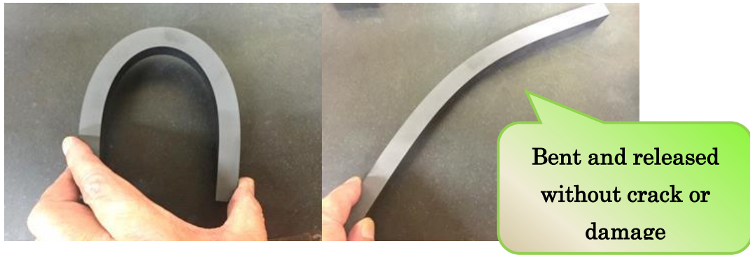
Picture 2.: Damping materials bent and straight crack
