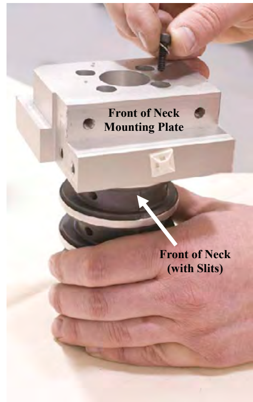
Figure 19. Assemble molded neck to neck mounting plate
