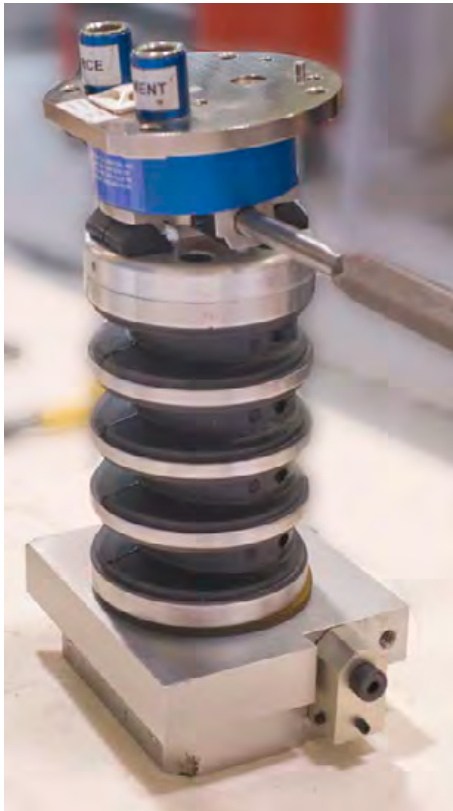
Figure 26. Align brass nodding joint washers with holes
