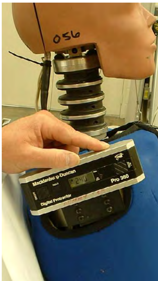
Figure 46. Adjusting the SID-IIIsD in the fore/aft plane
