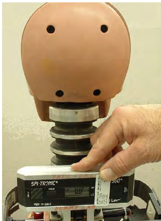
Figure 64. Adjusting the SID-IIsD in the lateral direction for iliac certification test
