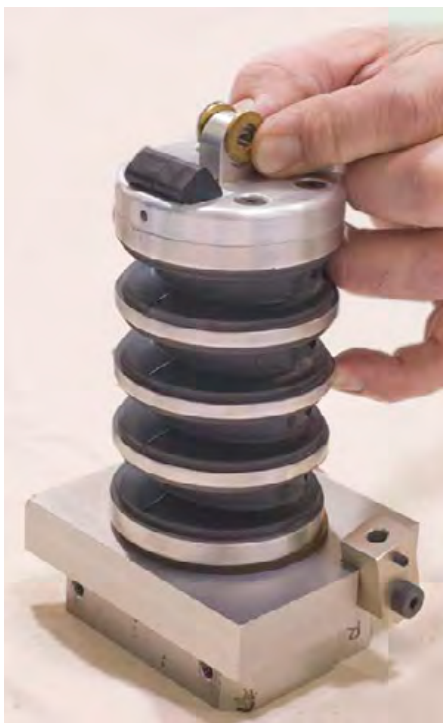
Figure 24. Install brass nodding joint washers
