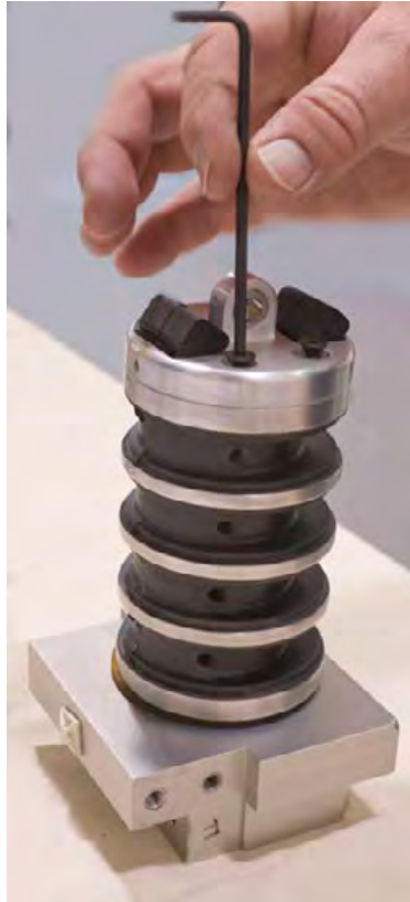
Figure 22. Reinstall neck nodding joint assembly
