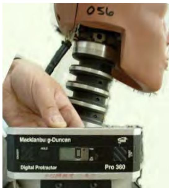
Figure 63. Adjusting the SID-IIIsD in the fore/aft plane for iliac certification test
