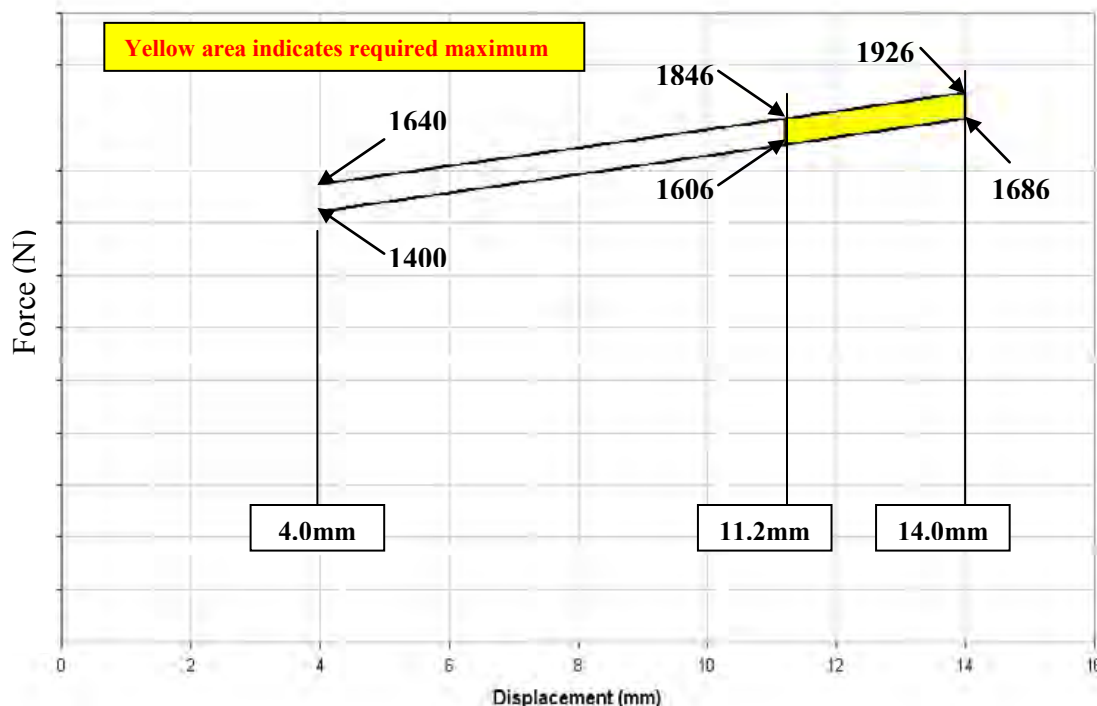
Figure 55. Corridor for pelvis plug certification test
