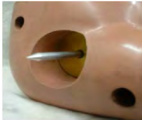
Figure 3. Threaded cylindrical tool installed at acetabulum
