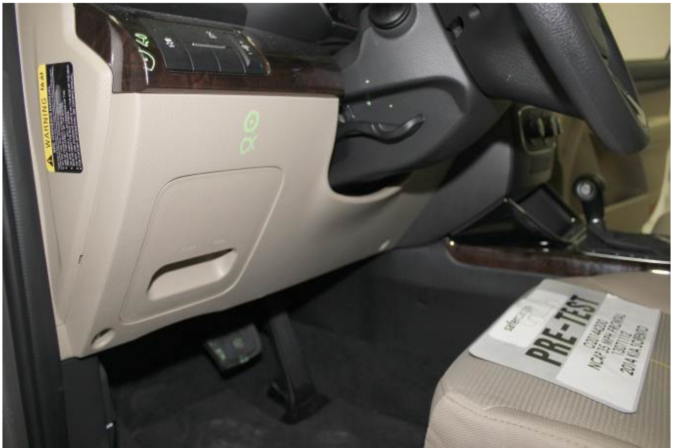
Pre-Test Driver's Side Knee Bolster (without dummy)
