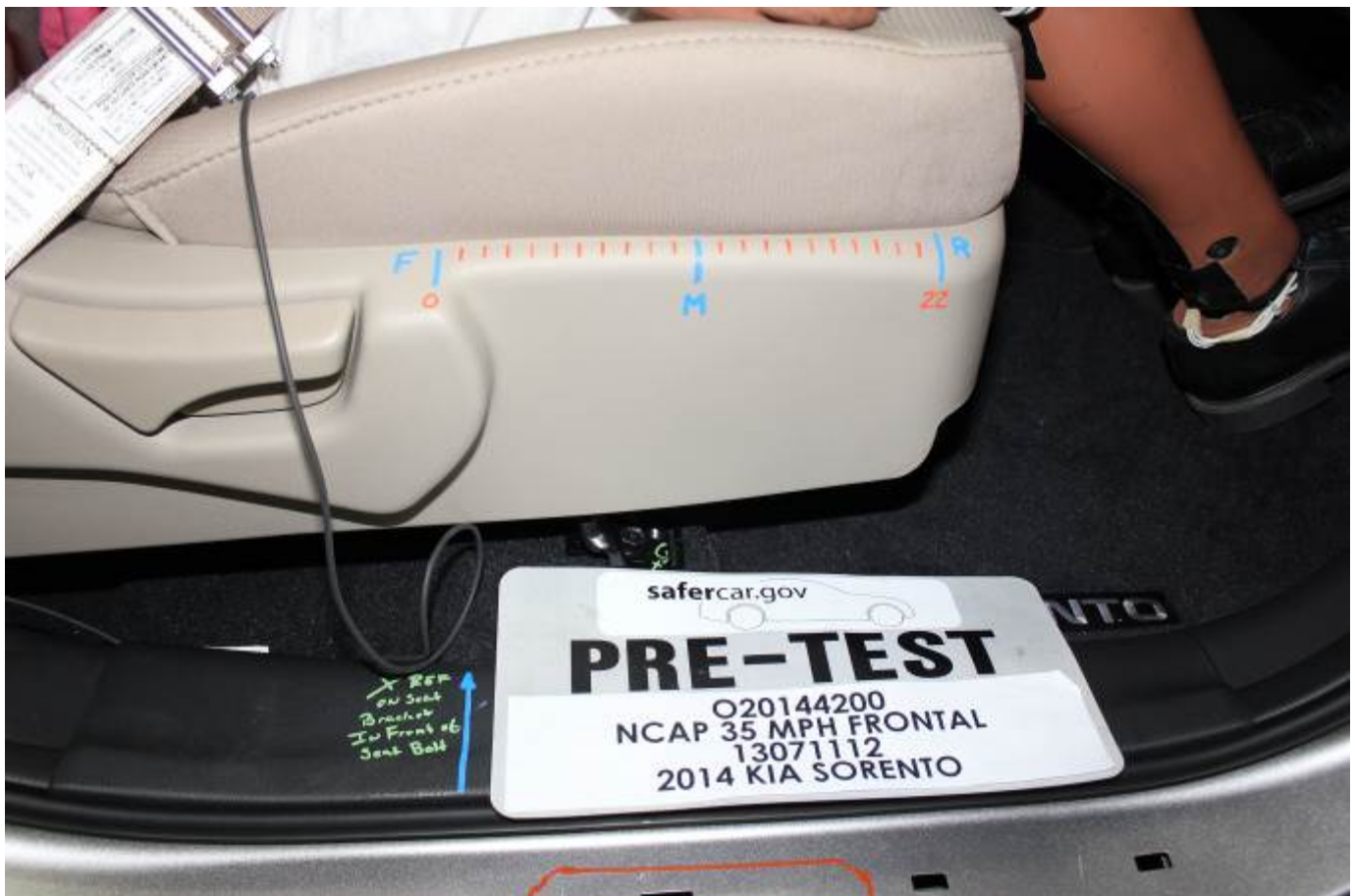
Pre-Test Passenger's Seat Fore-Aft Markings
