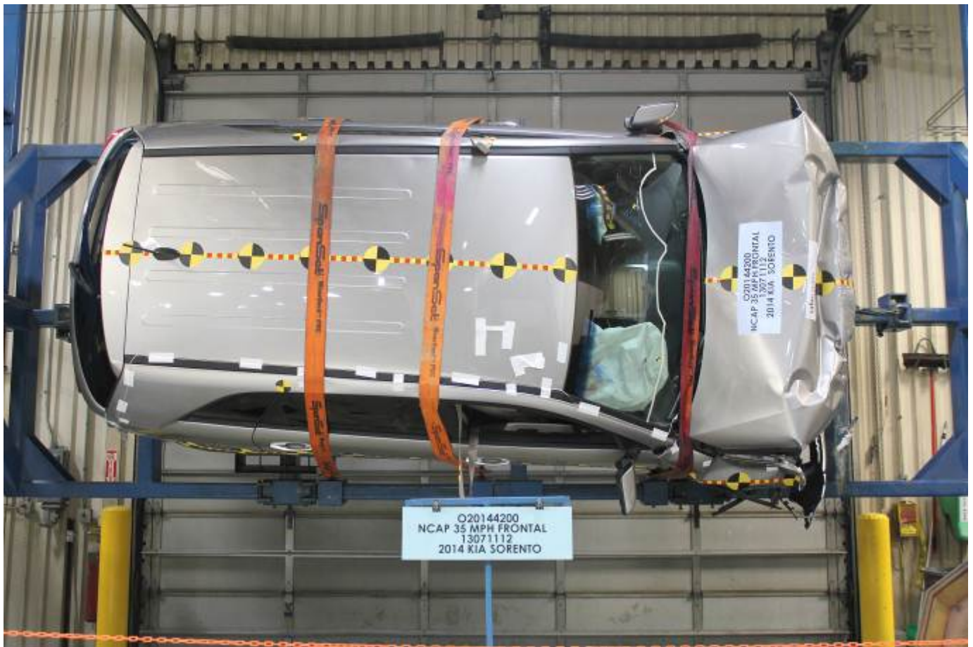
Vehicle at 270° on Static Rollover Device
