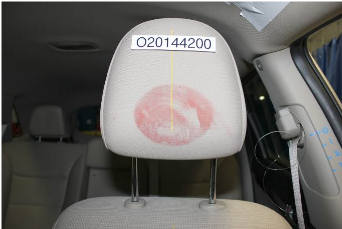
Post-Test Driver Dummy Contact with Headrest
