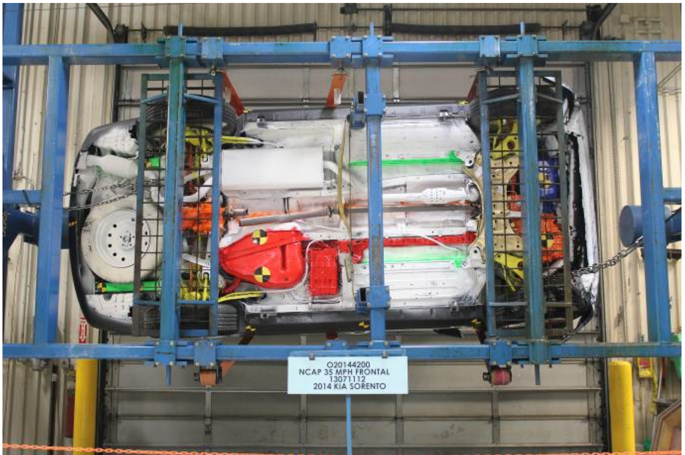
Vehicle at 90° on Static Rollover Device
