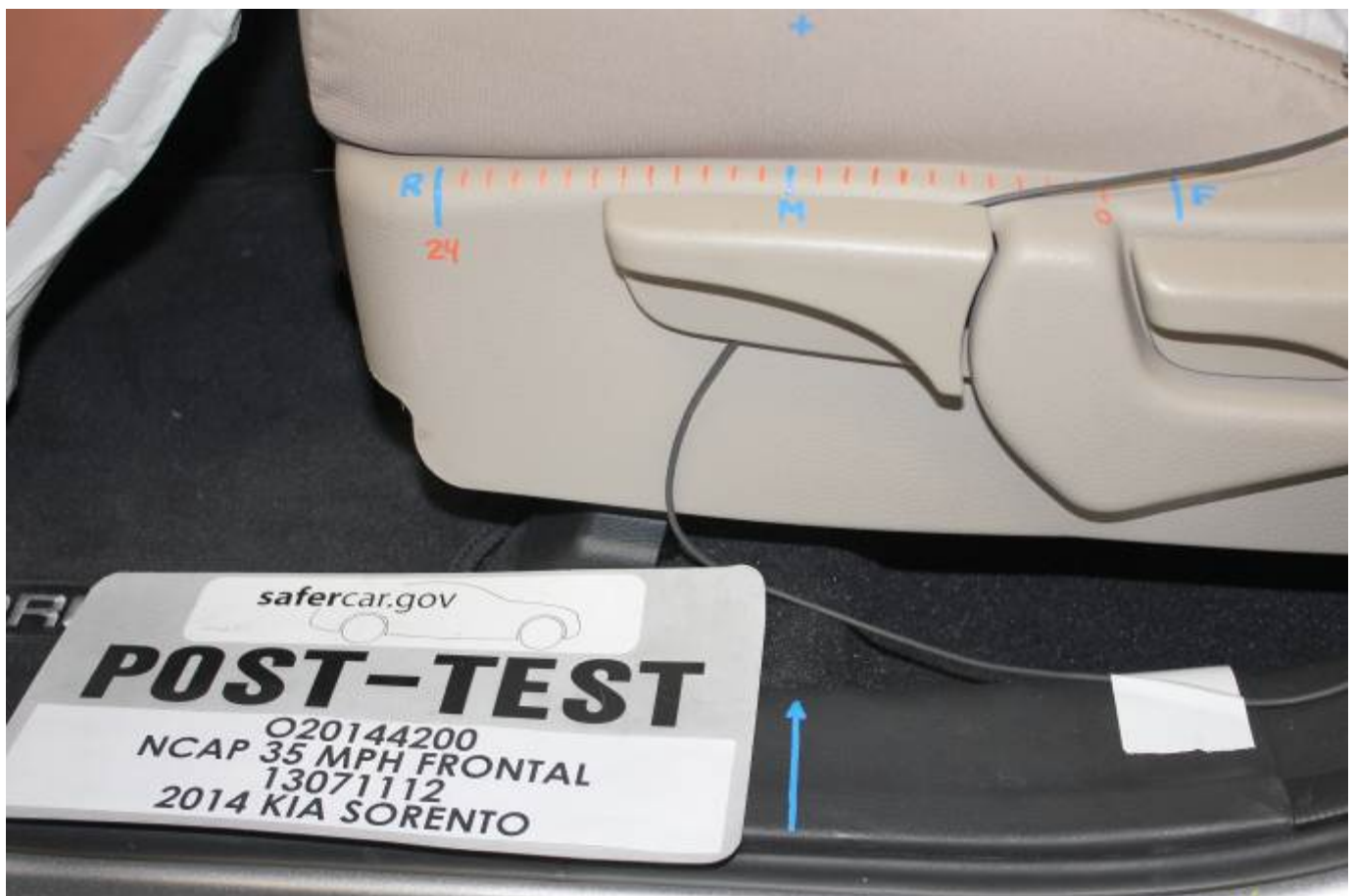
Post-Test Driver's Seat Fore-Aft Markings
