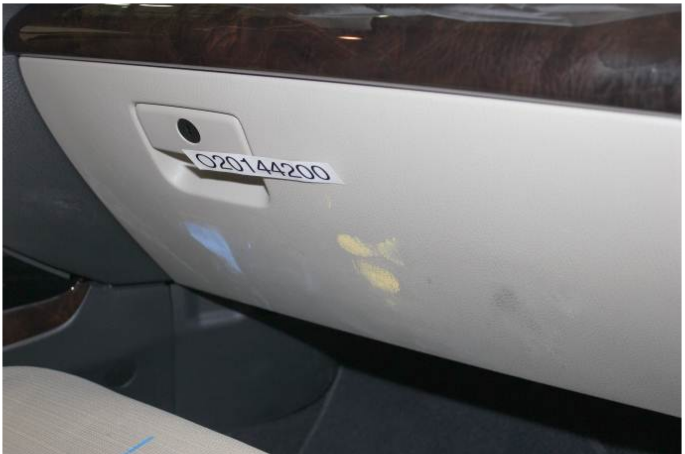
Post-Test Passenger Dummy Contact with Glove Box
