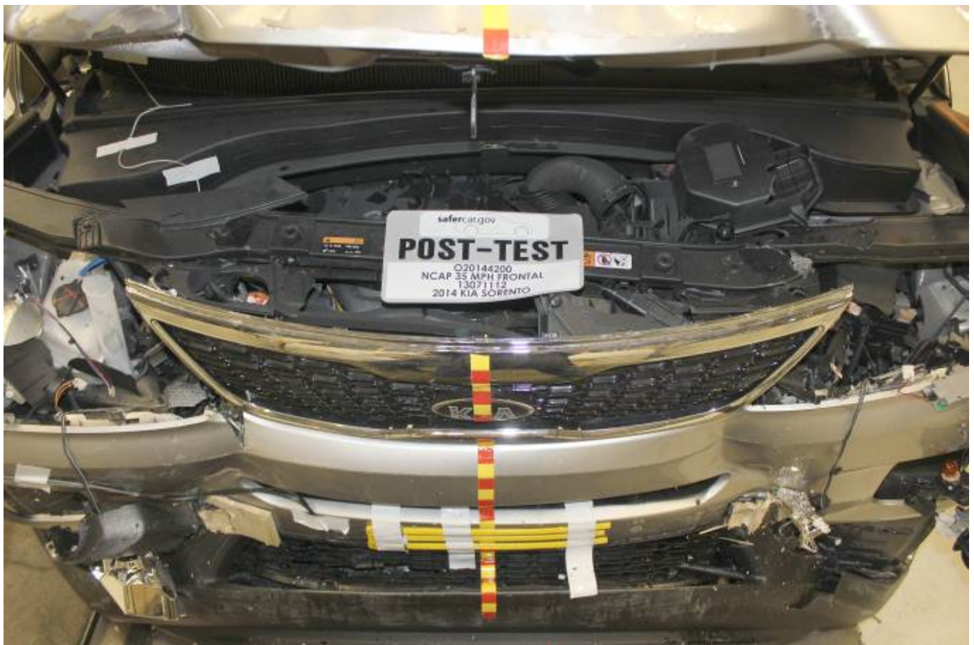
Post-Test Engine Compartment View
