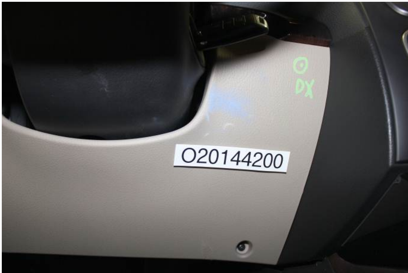
Post-Test Driver Dummy Contact with Knee Bolster
