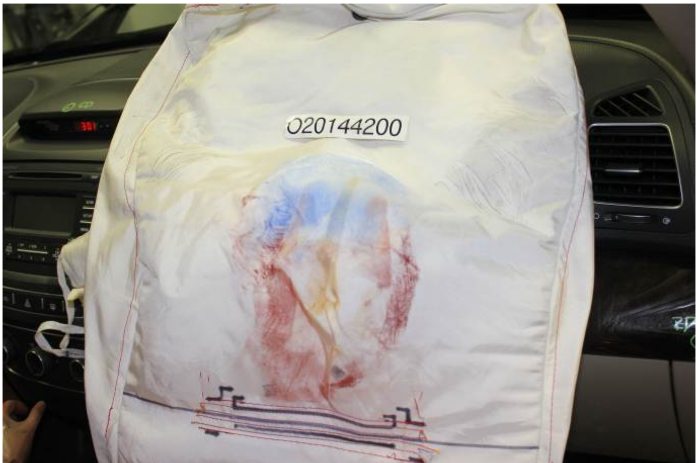
Post-Test Passenger Dummy Contact with Airbag
