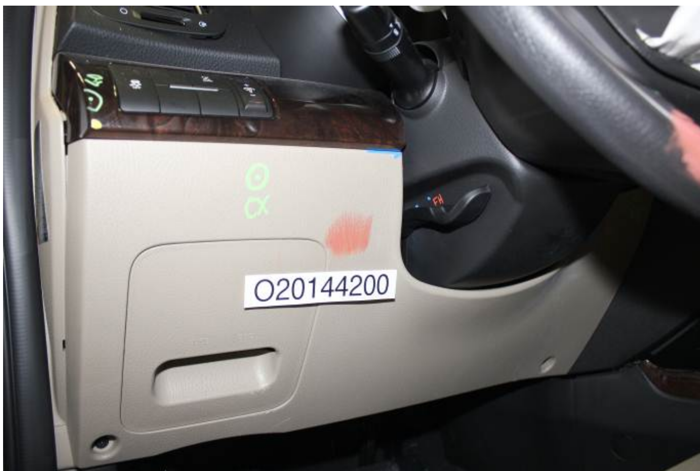
Post-Test Driver Dummy Contact with Knee Bolster
