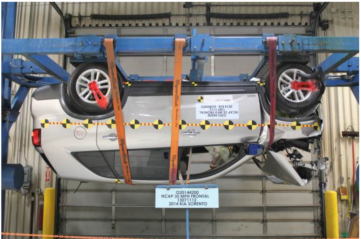
Vehicle at 180° on Static Rollover Device
