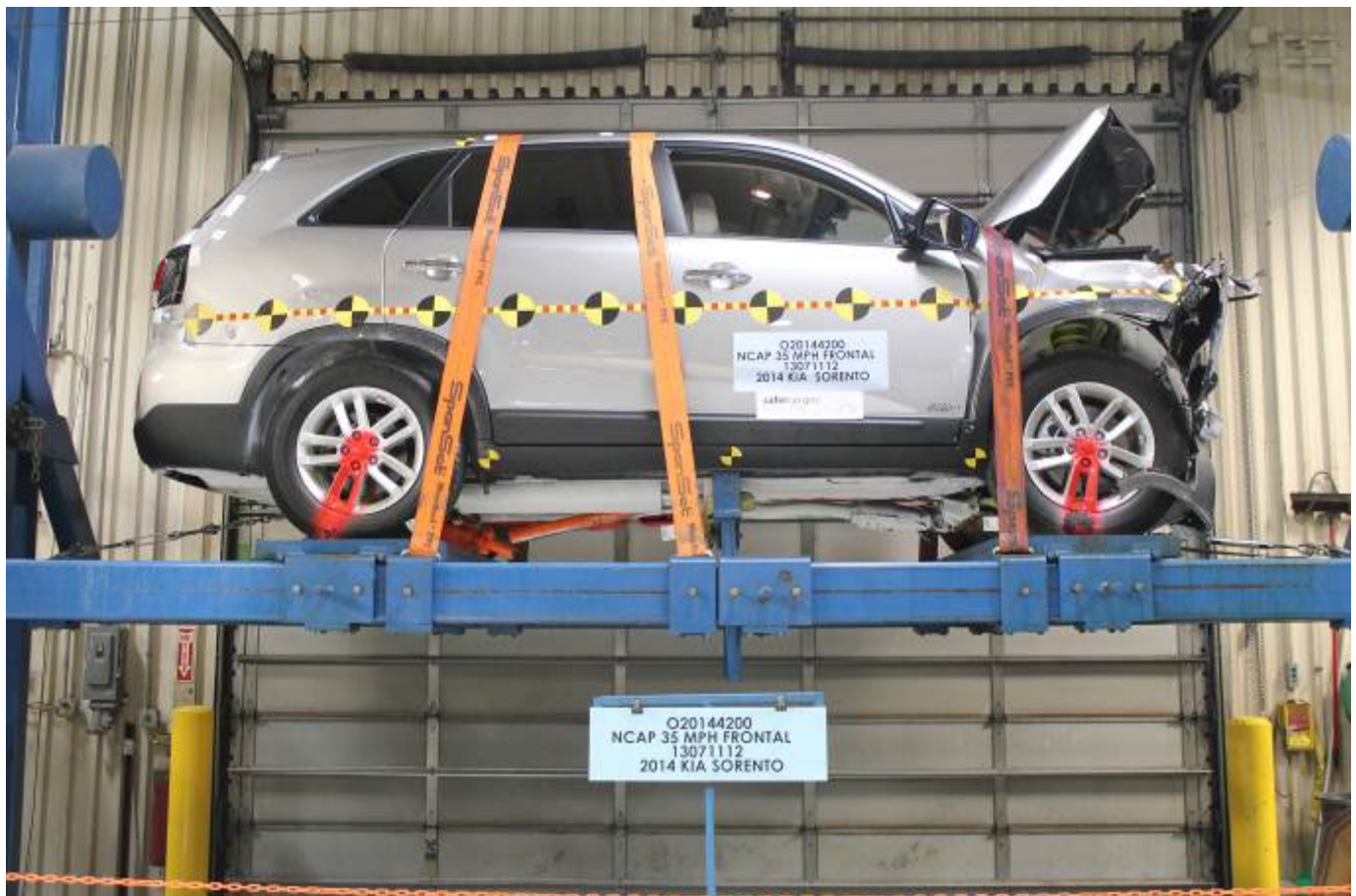
Vehicle at 0° on Static Rollover Device
