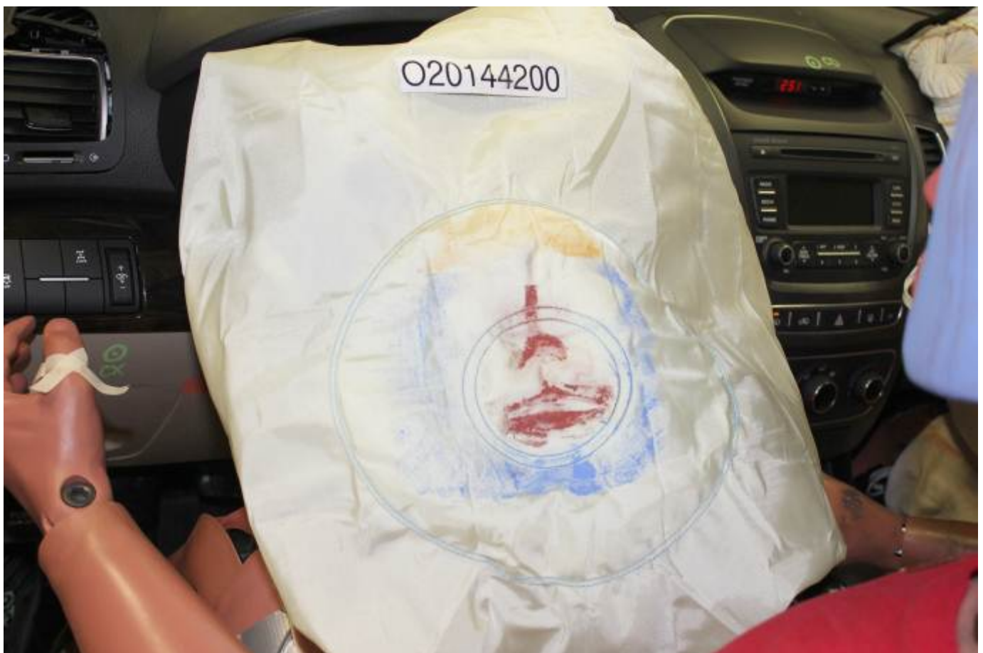
Post-Test Driver Dummy Contact with Airbag
