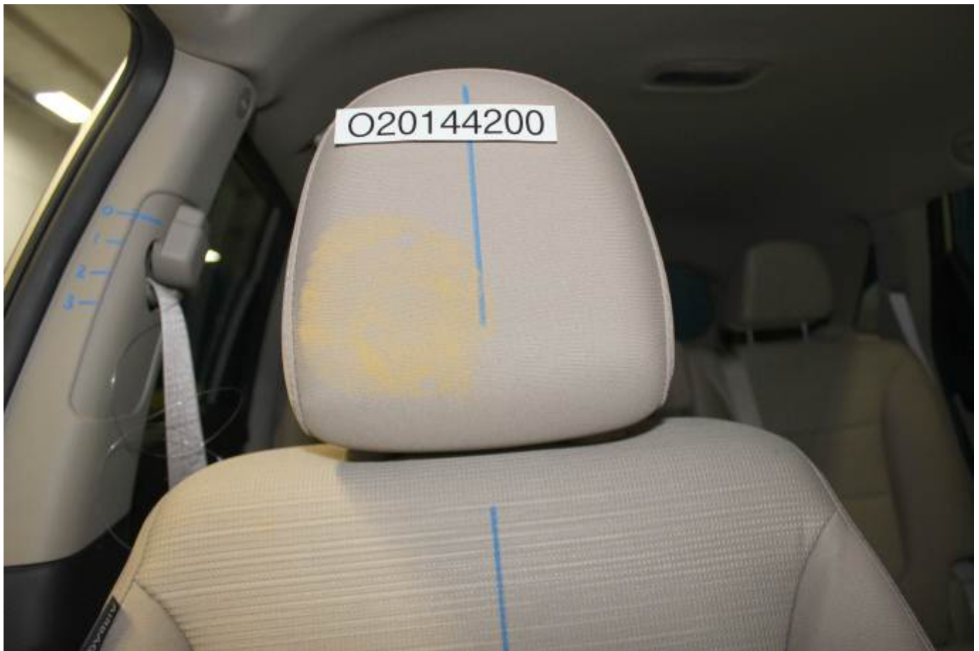
Post-Test Passenger Dummy Contact with Headrest
