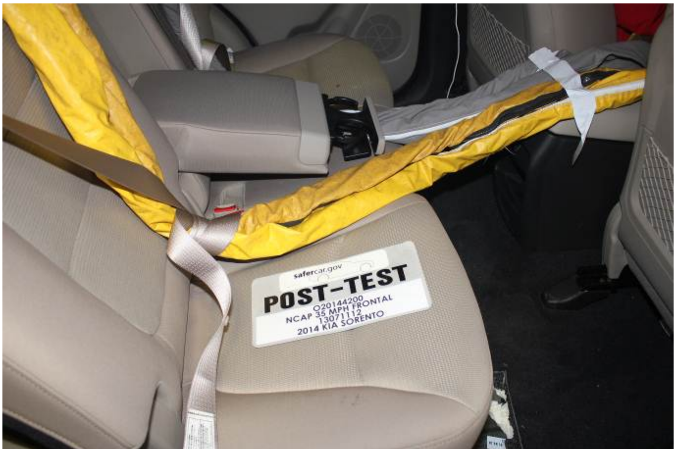
Post-Test Dummy Cable Routing
