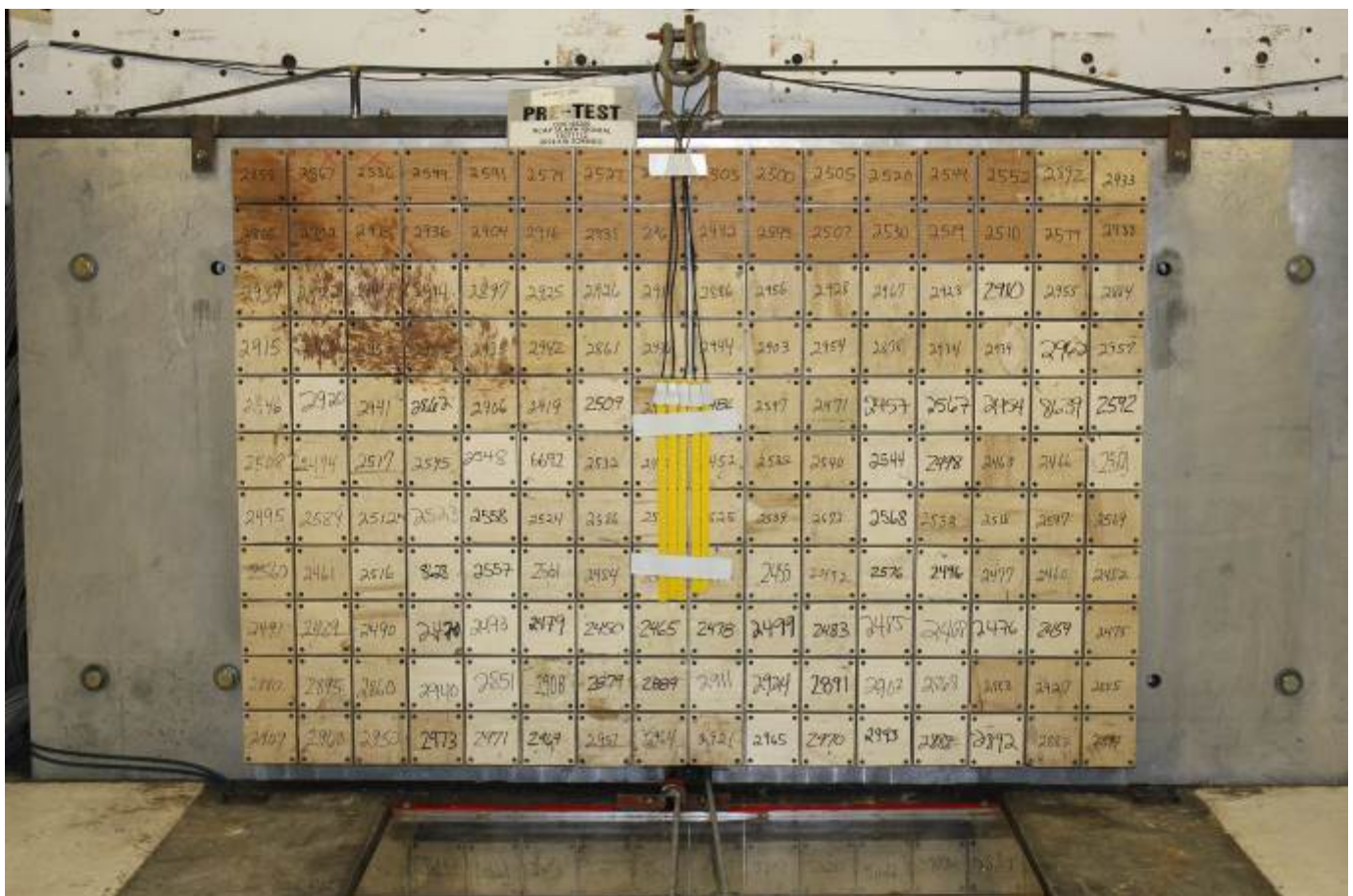
Load Cell Wall
