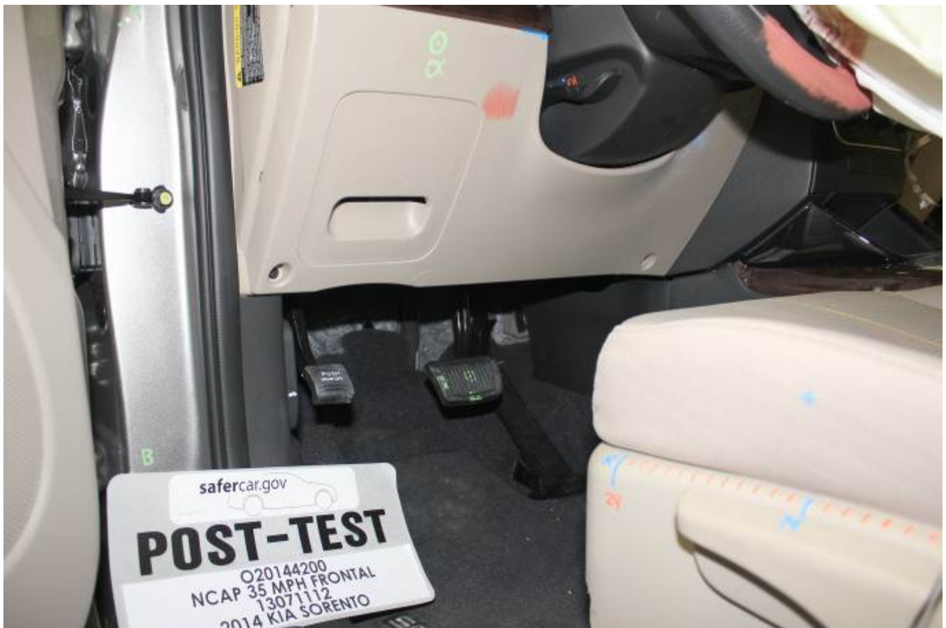
Post-Test Driver's Side Knee Bolster (without dummy)
