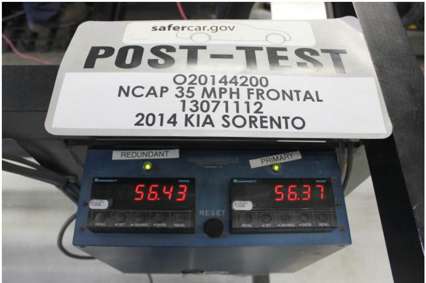
Post-Test Speed Trap Read-Out
