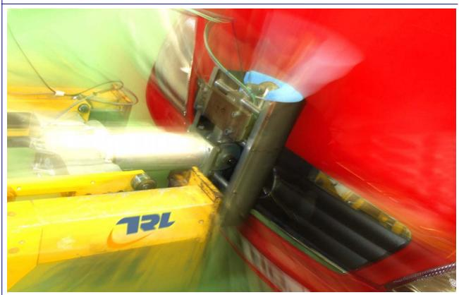
This impactor satisfies the requirement for sub-system testing of the bonnet/hood leading edge of all vehicles to GTR No. 9, the Commission Regulation (EC) No. 631/2009, EEVC WG 17 and EuroNCAP. It has also successfully performed tests into bull bars and high bumpers.
