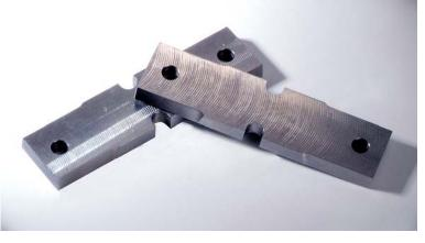
The Lower Legform Impactor uses deformable steel elements to provide the required knee bending response when testing to GTR No. 9, EC 621/2009, EuroNCAP, ANCAP and KNCAP.
