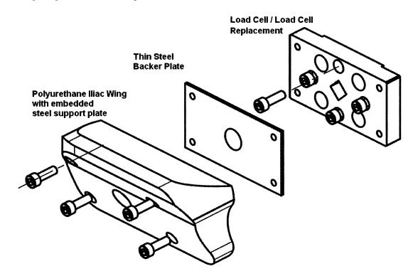
Figure 1: Alignment of iliac wing, backer plate, and load cell/replacement<sup>16</sup>
