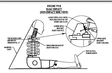
\* ALTERNATIVELY, A MATERIAL WITH A MAXIMUM STATIC BREAKING STRENGTH OF 311 N (70 LB) MAY BE USED TO SUPPORT THE DUMMY IN POSITION
